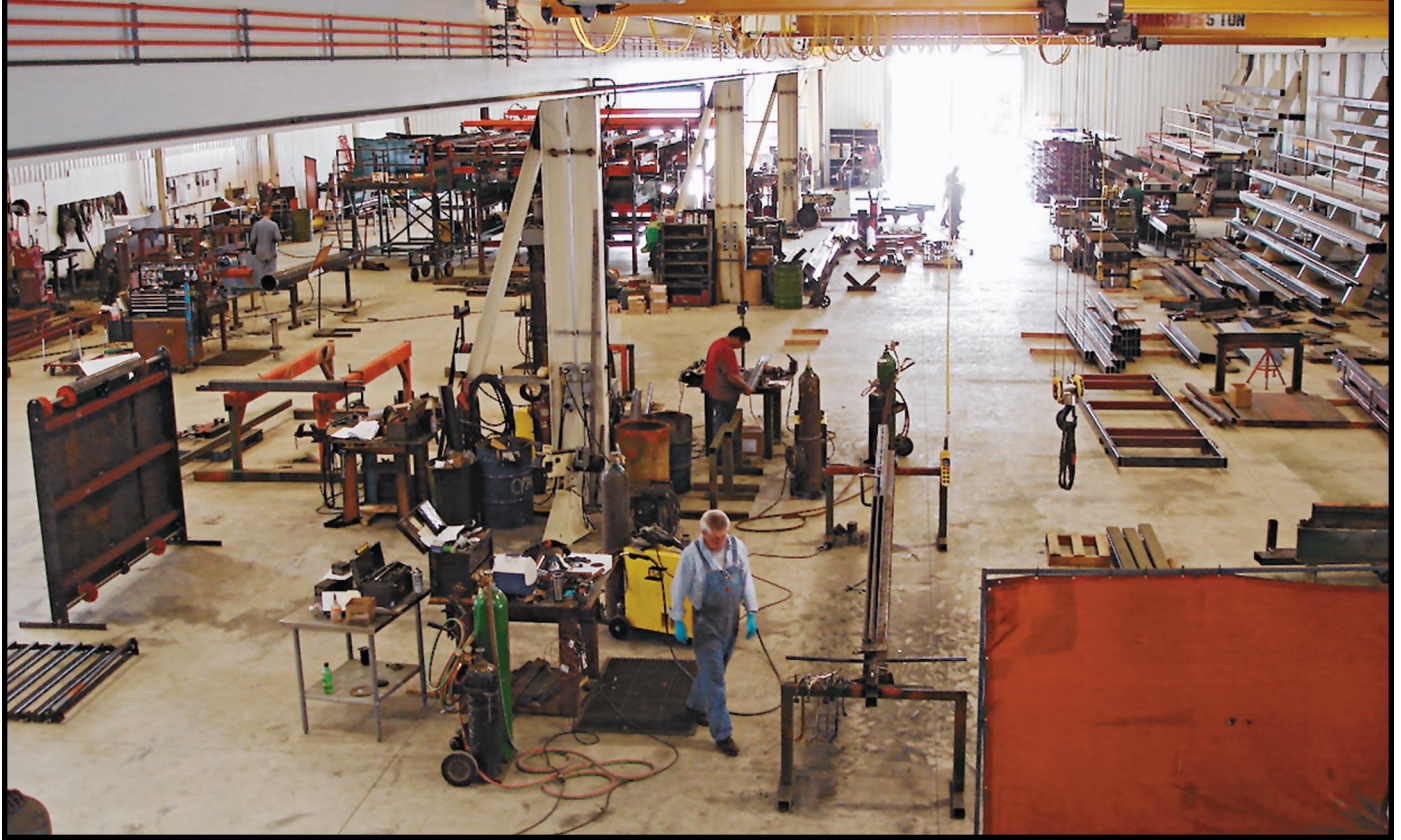
All MoCo Engineering systems are fully wired and test-run at the plant, a practice that makes startups much easier.
